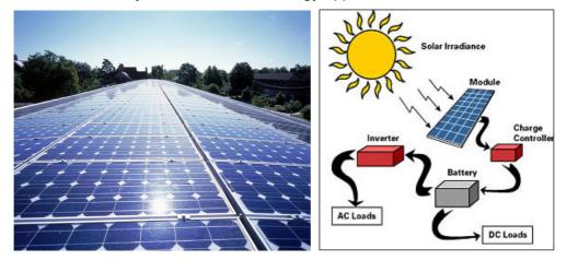
Figure 7 - Solar PV components
