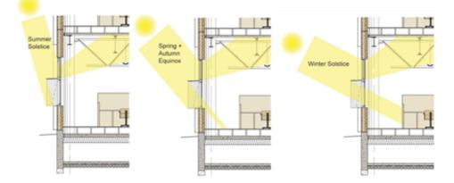
Figure 4 – Typical Daylight modelling design assessments
